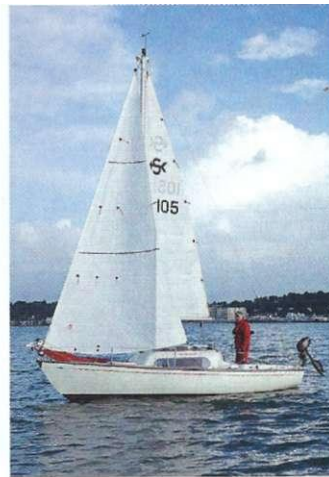
Heaving to in the conventional manner with the headsail aback
