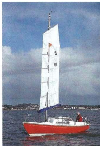
Stopping with a junk means letting the sheet go
