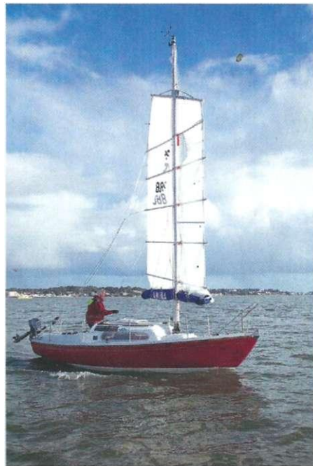
Reefing a junk means lowering the halyard to drop a panel (or as many as you want). Then take up the slack in the yard-hauling parcel
