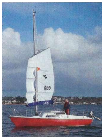
Lowering the junk sail means dropping the halyard...
